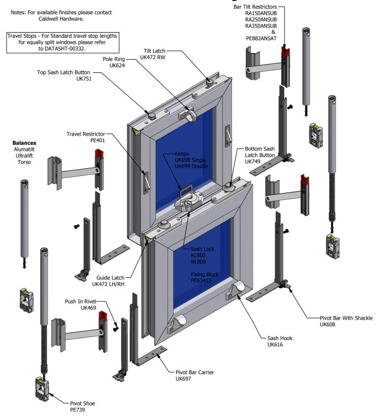
MINIMUM GAP BETWEEN SASH & FRAME MUST BE 3.5mm  $\pm \ ^{0.0}_{0.5}$
